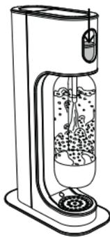
You can add more gas as desired by pressing the button again briefly once or twice. Release the button and wait until you hear another hiss as any excess pressure is discharged and the water bottle is vented.
