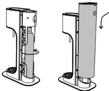
Slide the back section back into its guide grooves and push it down until the locking mechanism clicks back into place.
